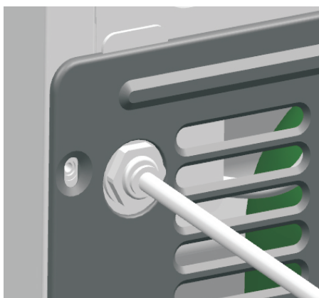
Step 3) Connect the PE soft tube
