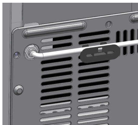
Step 6) Install the PE soft tube (Sketch map)
