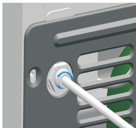
Step 4) Install the security clamp
